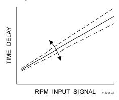
Adjusts the ratio of the governor speed setting signal to the time delay. This adjustment is only effective on the proportional time delay.
