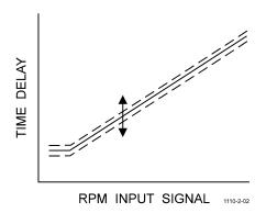
Adjusts independently the time delay over the entire range of governor speed setting signal. The base adjustment affects both the fixed and proportional time delay.
