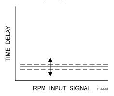
Adjusts, independently Ahead and Astern, the minimum time delay for low speed maneuvering. This adjustment has no effect on the proportional time delay.
