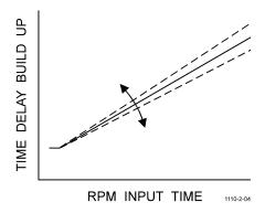
Adjusts the rate of build up of the proportional time delay. An optional fixed time delay build up adjustment can also be provided.
