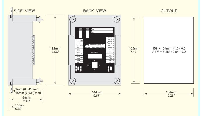
Mounting hardware is included with each unit and consists of 4 knurled thumb nuts and 4 clamps.
