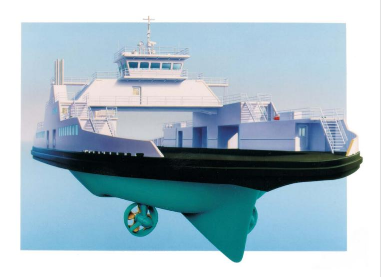
For British Columbia Ferry Corporation 110 meter (360 feet) Double-Ended RO-RO/Passenger CENTURY CLASS FERRY built by Allied Shipbuilders Ltd.
