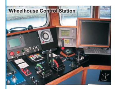
The propulsion control system for the M/V Stikine is a dual-mode PMC D-MaC (Digital-Marine Control). The controls include hybrid combinator mode and split mode for control of the two Cat 3512 engines driving Hundested controllable pitch propellers.
